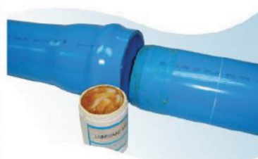
STEP 4 Apply lubricant to the spigot end and approximately mid-way back to the reference line.
