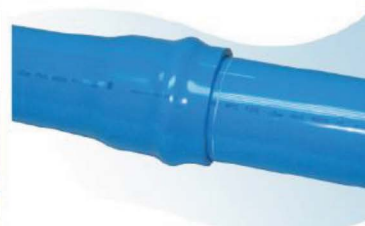
STEP 5 Insert the spigot end into the socket and apply steady pressure until the spigot slips through the rubber ring. Insert pipe until the reference line is just visible at the face.
